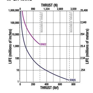
NOTE: The L<sub>10</sub> expected life of a ball screw linear actuator is expressed as the linear travel distance that 90% of properly maintained ball screws manufactured are expected to meet or exceed. This is not a guarantee and this graph should be used for estimation purposes only.
